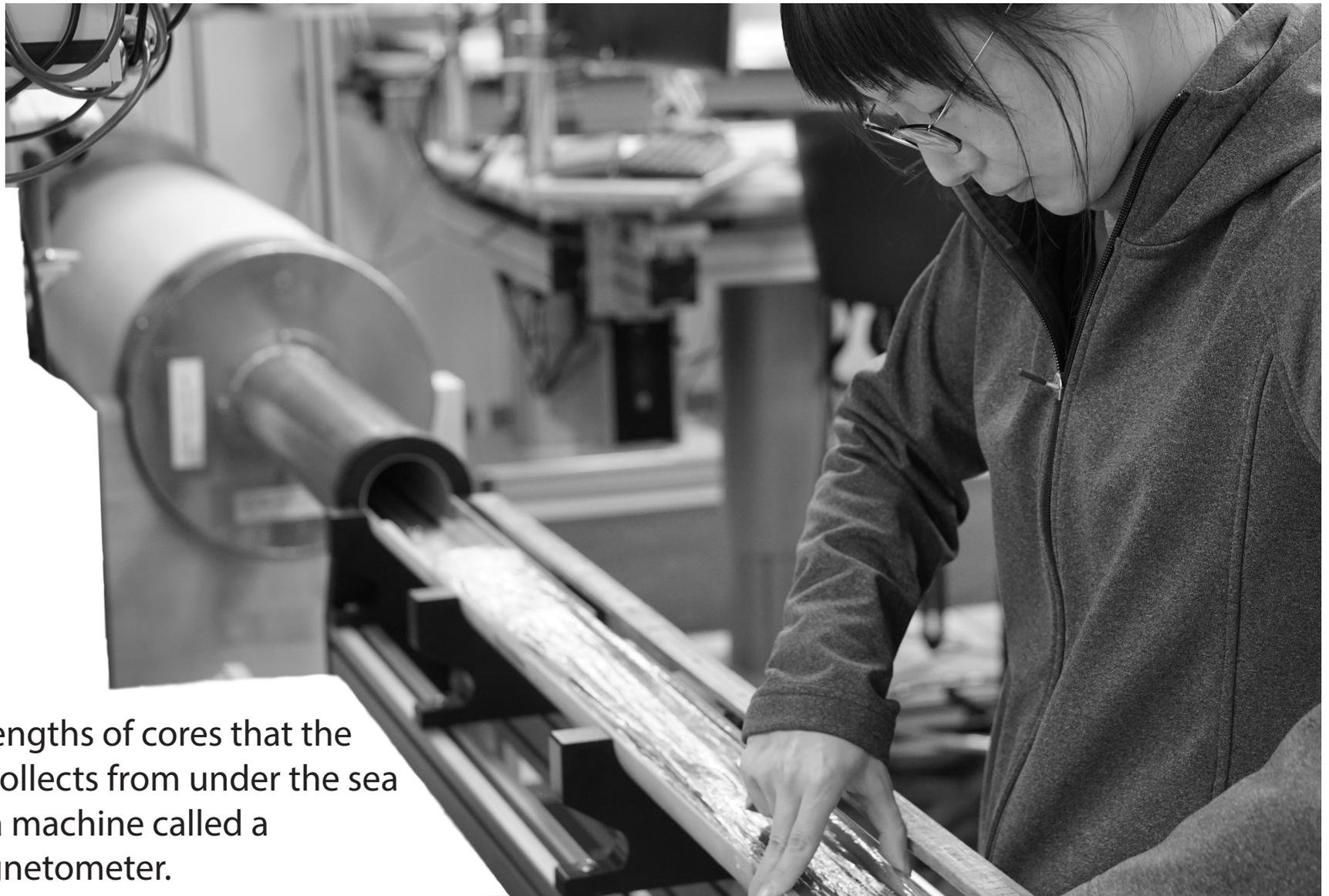
Saiko puts the lengths of cores that the *JOIDES Resolution* collects from under the sea floor into a machine called a magnetometer.
