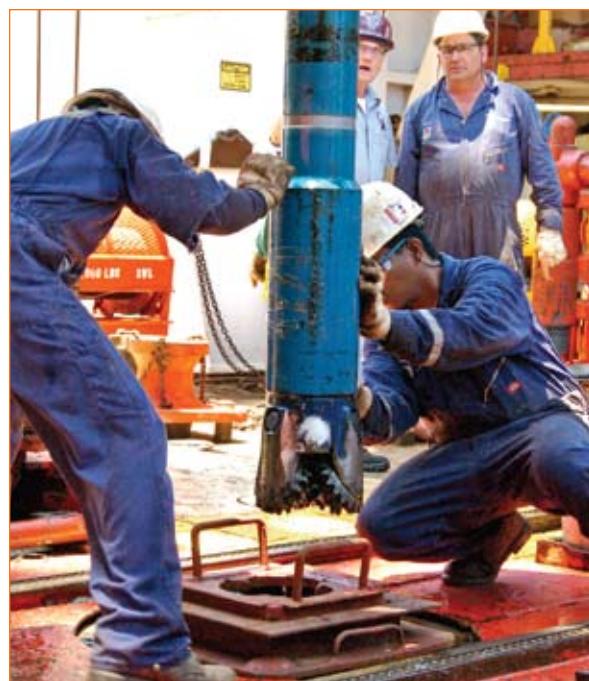
Roughnecks aboard the JOIDES Resolution guide the drill bit through the rig floor and towards the seafloor to begin drilling for cores. (image courtesy IODP-USIO)
