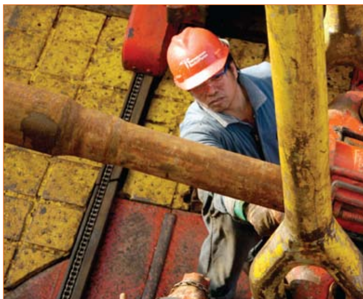
A roughneck on the JOIDES Resolution helps guide the drill pipe using the drawworks during the pipe tripping process. (image courtesy IODP-USIO)
