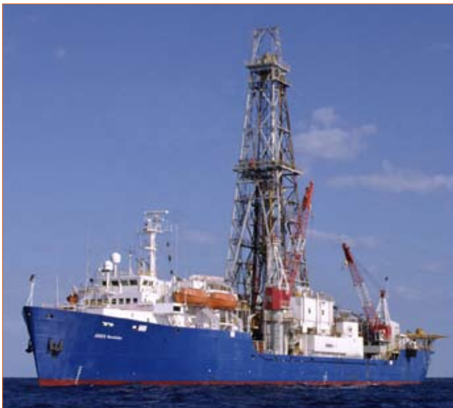
The scientific drilling vessel, JOIDES Resolution, is a floating laboratory which has collected cores worldwide.
