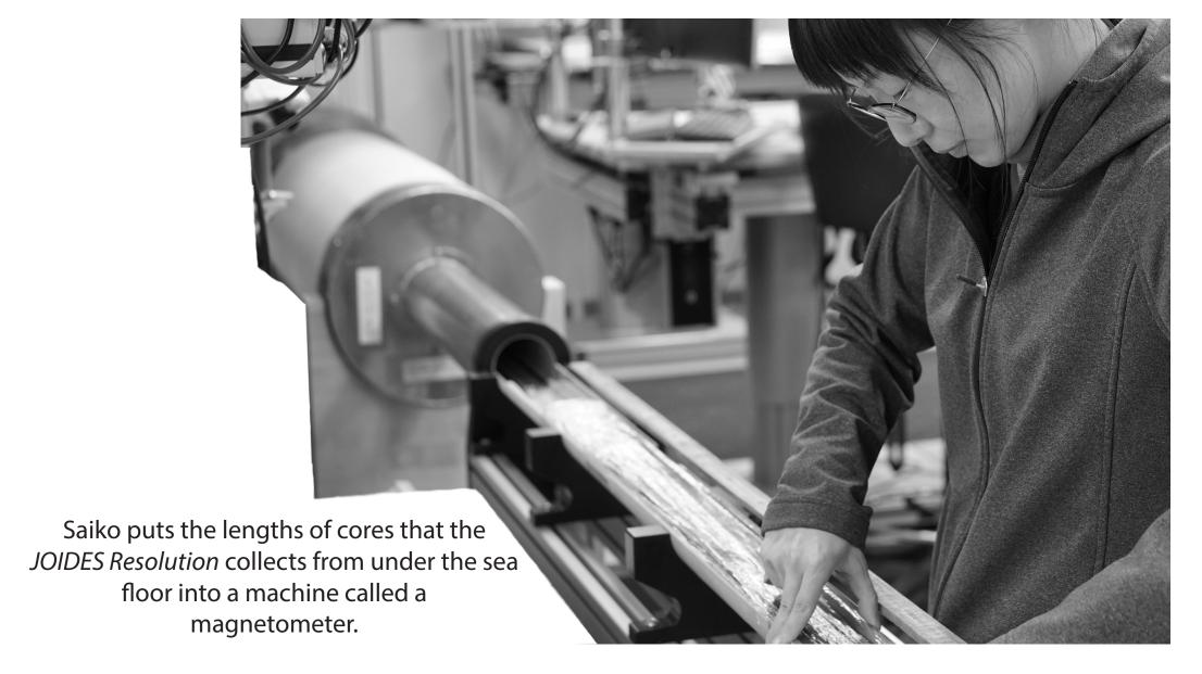
The magnetometer uses the magnetic minerals in the mud and stone to figure out which direction the magnetic field was pointing when that mud and stone was layered on the bottom of the ocean.
