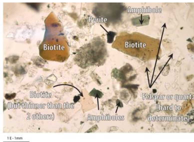
Example of a smear slide made on board during Expedition 362 showing typical minerals of plutonic rocks (Smear-slide 362U1480E-7H-1-SED-99039601)
