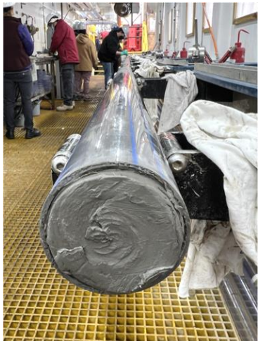
A close-up of sediment in a freshly retrieved EXP 400 core (Michelle Pratt)
